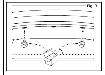
3) Push trunk trim back up, reinstall (2) outer push pins and discard 3rd push pin
