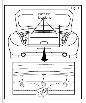
1) Remove (3) push pins from package shelf using a flat head screw driver and save to reuse.
