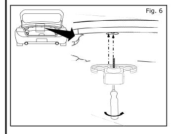
8) With shopping bag hook in stowed position, insert screw, align with jack nut and anti-rotation hole and fully tighten.
